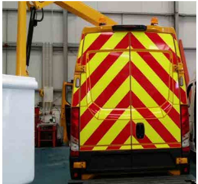
Picture 1: Example of high-visibility vehicle markings in the form of rear chevrons.
