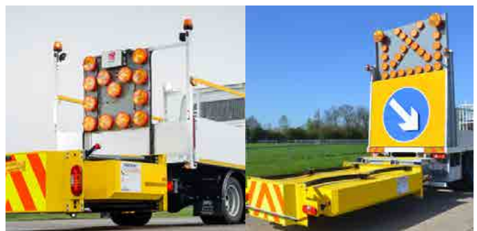
Pictures 2 and 3: Examples of vehicles fitted with impact protection used to alert other road Users of vehicles working from or immediately next to the road, provide appropriate information to drivers and to reduce the severity of injury should a road User collision with a works vehicle occur.
